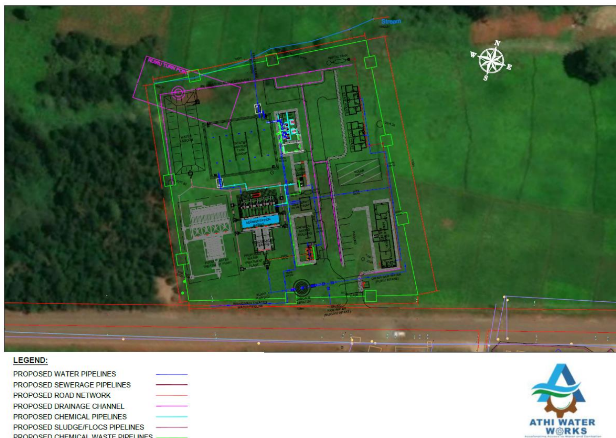
Figure 2-5 New water treatment plant indicative layout - Githunguri
