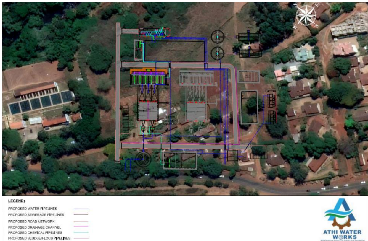
Figure 1-6 New WTP 70MLD / Train Footprint
