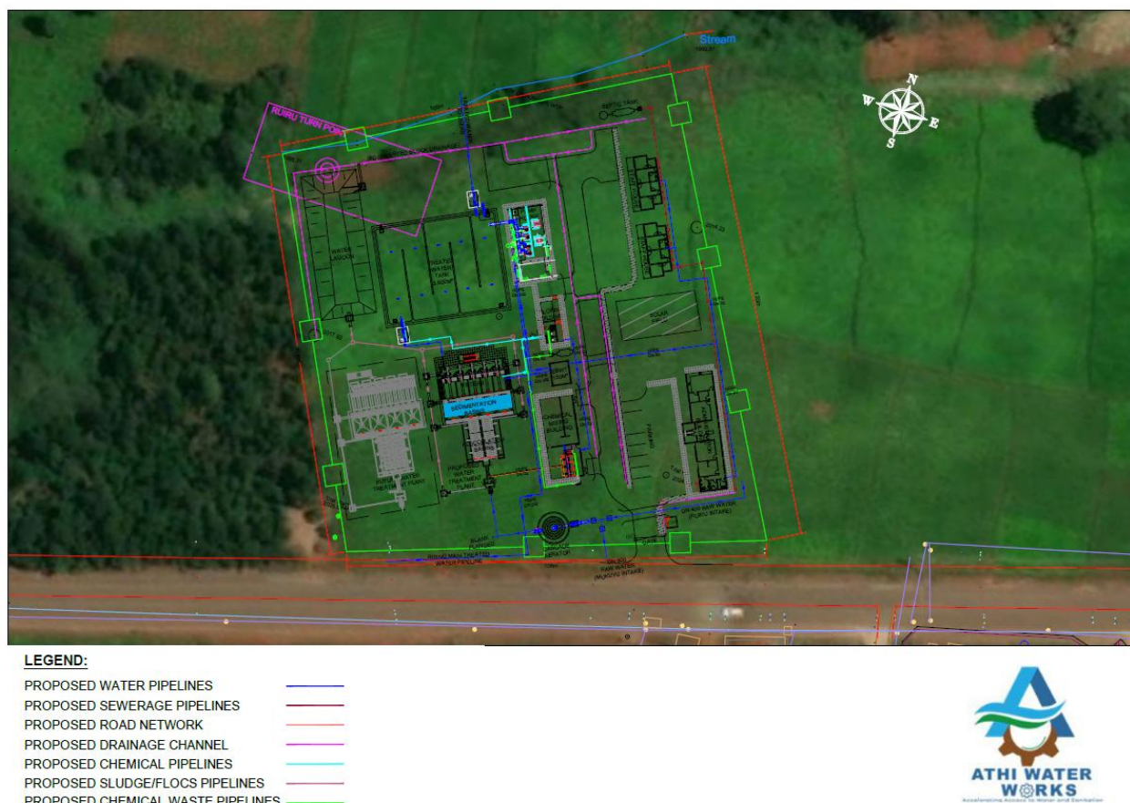
Figure 2-5 New water treatment plant indicative layout - Githunguri
